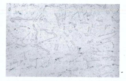
Fig. 3 Photomicrograph showing type 309 parent metal away from weldment area of annealing inner cover cone section. Sigma phase and some fine carbides can be noted in the austenitic matrix, Etchant, mixed acids, Magnification 500X. (Reduced 10%.)
