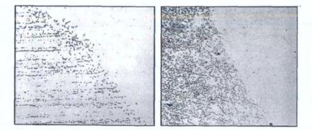
Fig. 9 Fusion zone between 309 parent metal (left hand side of 9A) and RA 330-04 bare wire. The deposit metal is fully austenitic while the ferrite content of the base metal as determined by a Magne-Gage was one percent in the as-welded condition. After signatizing (9B) about 20% sigma can be noted in the base metal (left hand side of 9B) while the weld deposit metal has remained fully austenitic. ~ Magnification 235X (Reduced 10%). Etchant, Vilella's.
