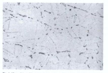
Fig. 4 View of type 309 parent metal under weld bead of annealing inner cover cone section. Note difference in darkness of sigma phase along with lesser amount present than in Fig. 3. Etchant, mixed acids. Magnification 500X. (Reduced 10%.)
