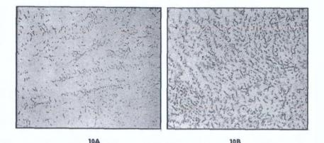
Fig. 10 Type 309-16 weld deposit metal in the as-welded condition and in the sigmatized condition (10A and 10B, respectively). Magnification 235X (Reduced 10%). Etchant, Vilelle's.
