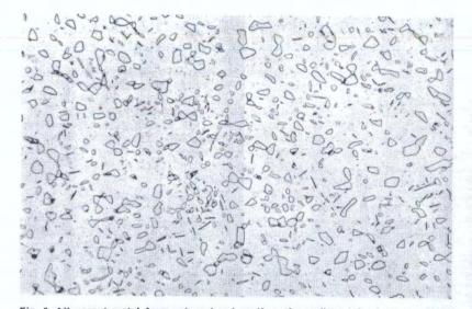
Fig. 5 All parent metal from return bend portion of a radiant tube from an aluminum ingot heating facility after four years of service. The 500X micrograph shows sigma phase present in an austenitic matrix. Etchant, mixed acids. (Reduced 10%.)
