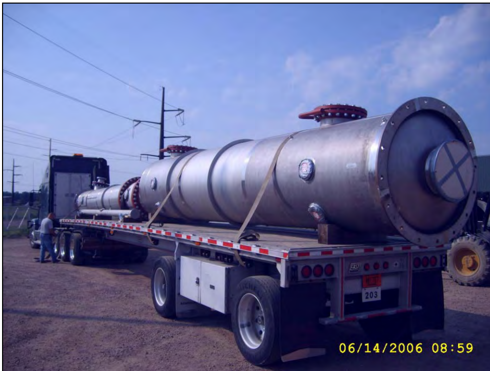
Fig. 27 2507 super duplex vessels used in the biodiesel production
