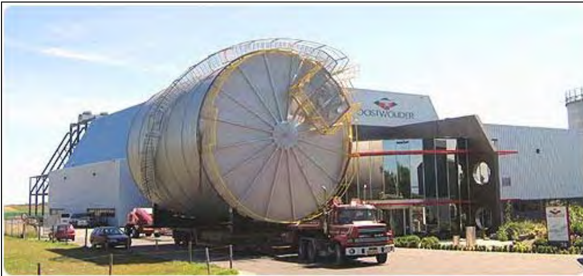
Fig. 20 LDX 2101 was used by Oostwouder Tank- & Silobouw BV of the Netherlands to fabricate these tanks used in the production of biodiesel for a project named Greenmills [6]
