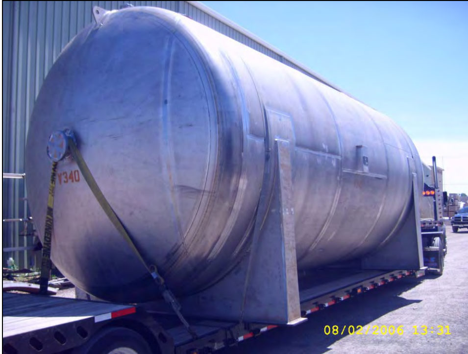
Fig. 26 Biodiesel reactor vessel fabricated from 2507 super duplex stainless
