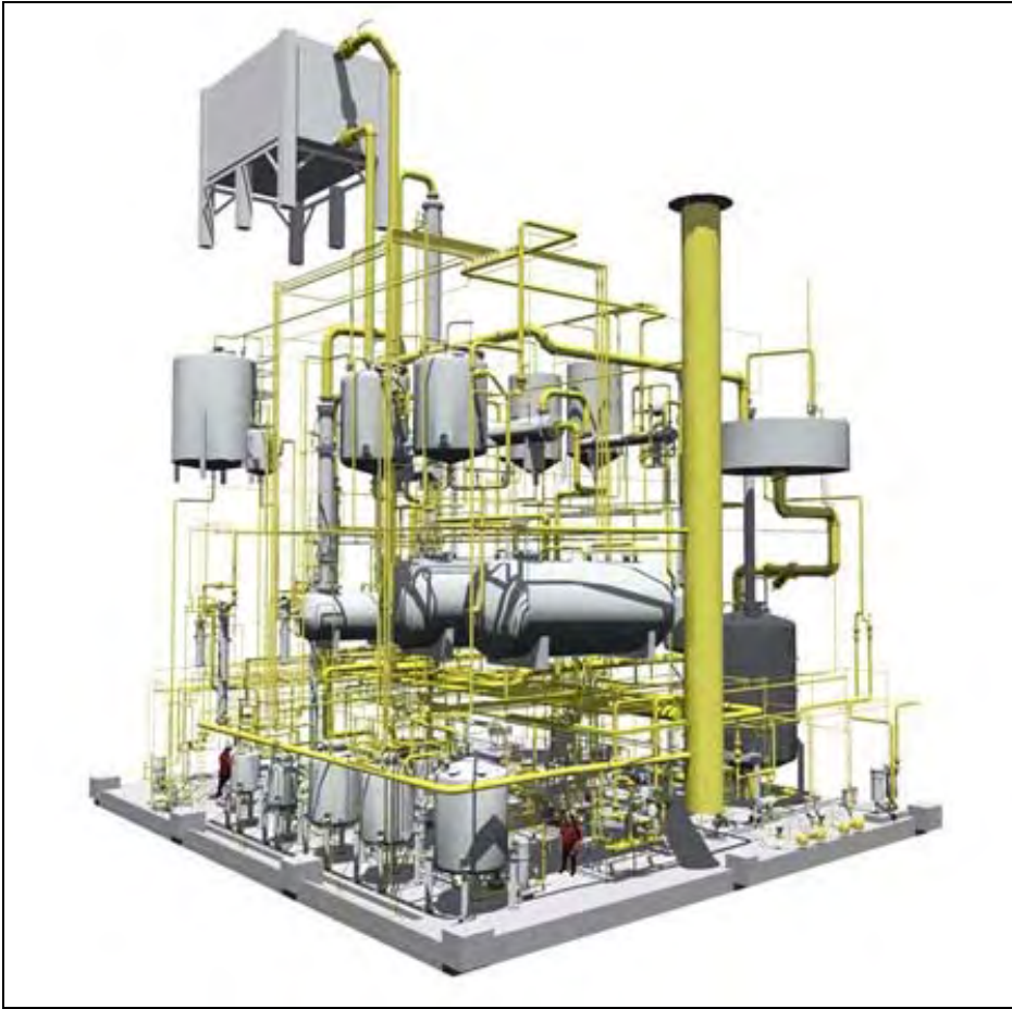
Fig. 25 Schematic of a biodiesel process facility. The vertical tanks on the second level have been fabricated from 2507 superduplex.
