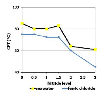
Figure 1. Effect of nitride level of UNS S32760 alloys on corrosion resistance in an ASTM G48 Method A test and in simulated seawater
