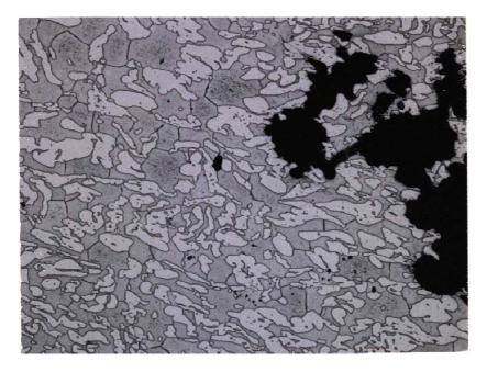
Figure 2. Photomicrograph of a UNS 32760 Alloy showing selective corrosion attack of the ferrite phase as a result of nitride precipitation.
