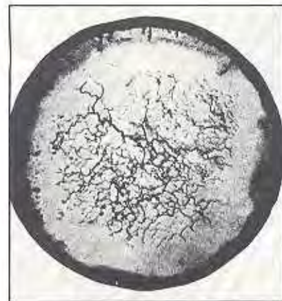
Fig. 3 Typical thermal fatigue damage after repeated quenching.
