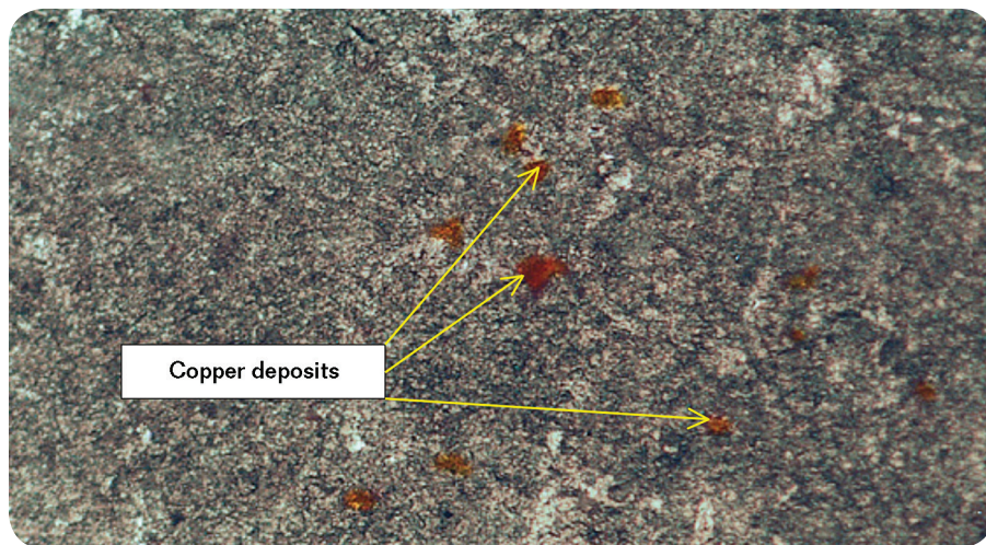
FIGURE 1 Copper deposits on superduplex SS after three weeks in aerated seawater plus 50 mg/L cupric ions.
